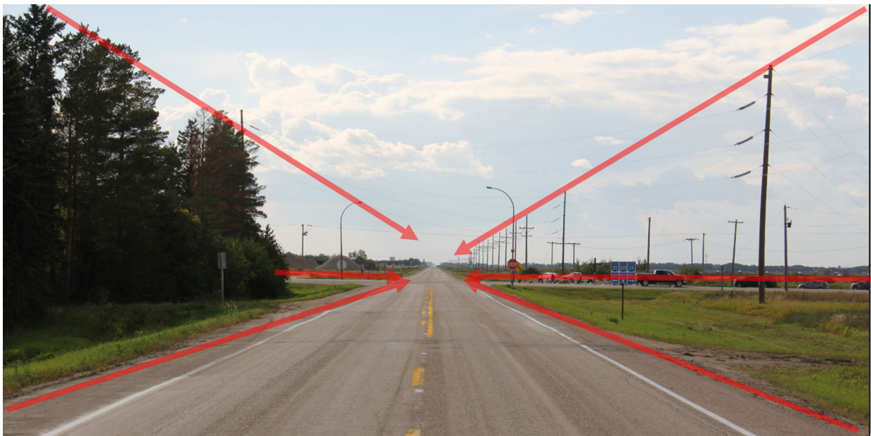
Figure 7-1: Tunnel Vision on Westbound Highway 335
